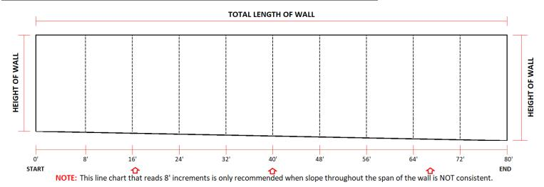
INSTRUCTIONS: (Recommended tools; 4' to 6' Level, both 100' Tape and 25' Tape, Pencil and paper to record measurements)
