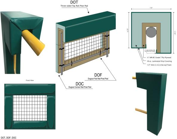
Vinyl Covering: 18 oz. per sq/ yard laminated vinyl, unbalanced coating. Fabric: 1000 Denier Polyester Basic Fabric, Tear Strength Test: Warp 100 lbs., Fill 315, lbs., Tensile Strength: Warp 300 lbs. Fill 300 lbs., Weft Insertion: 18x17, Superior UV inhibitors, Cold Crack: Minus 40 degrees Fahrenheit. Colors per manufacturer's standard selection, as selected by Architect.
